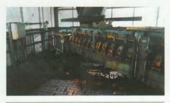
**Figure 1.** Before the upgrade, fugitive material required about 90 man-hours per week to safely clean and haul away.
