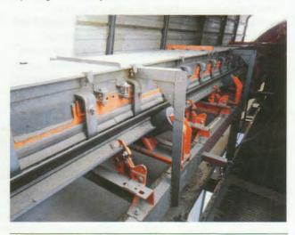
**Figure 3.** The project included upgraded transfer points to eliminate belt sag and improve sealing, as well as belt cleaning and alignment systems.
